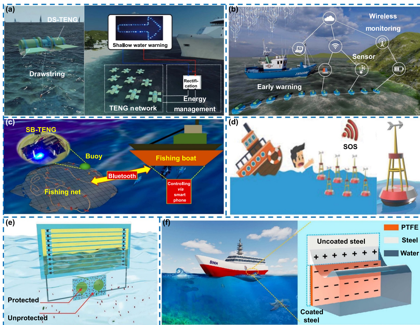
Figure 13. The applications of ocean navigation support. (a) The drawstring W-TENG used to provide warnings to ships to avoid stranding. Adapted from [178], with permission from Springer Nature. (b) The CE-TENG that can provide power for radar warning. Reprinted from [179], © 2023 Elsevier Ltd All rights reserved. (c) The smart buoy-TENG toward self-powered smart fishing net tracker. Reprinted (adapted) with permission from [180]. Copyright (2020) American Chemical Society. (d) The liquid–solid contact W-TENG in buoys. [181] John Wiley & Sons. © 2018 WILEY-VCH Verlag GmbH & Co. KGaA, Weinheim. (e) The achieve antifouling on wetted insulating surfaces. [182] John Wiley & Sons. © 2016 WILEY-VCH Verlag GmbH & Co. KGaA, Weinheim. (f) The W-TENG used to ship anti-corrosion. Reprinted (adapted) with permission from [42]. Copyright (2022) American Chemical Society.
